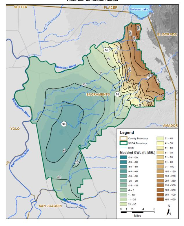
Figure 13: Groundwater Elevation Contour Map at the End of Simulation – Historical Calibration Model
