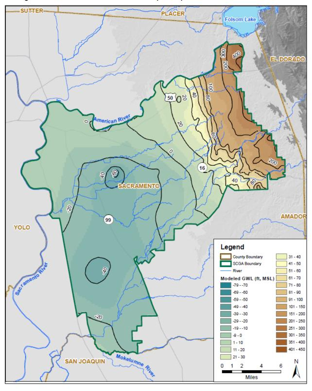
Figure 9: Groundwater Elevation Contour Map for September 1977 – 2030 Baseline Model
