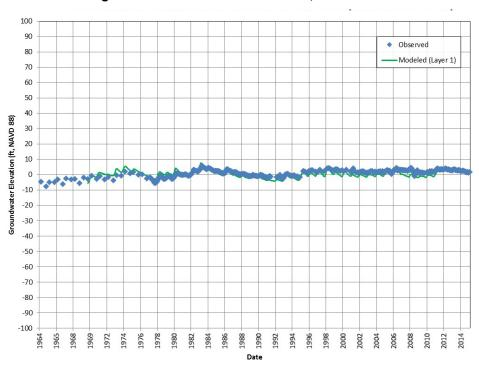
Figure 11c: Groundwater Elevation, Calibration Well 80
