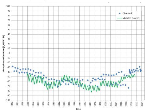
Figure 11g: Groundwater Elevation, Calibration Well 189
