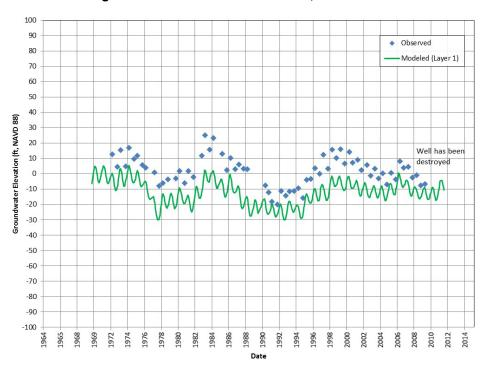
Figure 11e: Groundwater Elevation, Calibration Well 109
