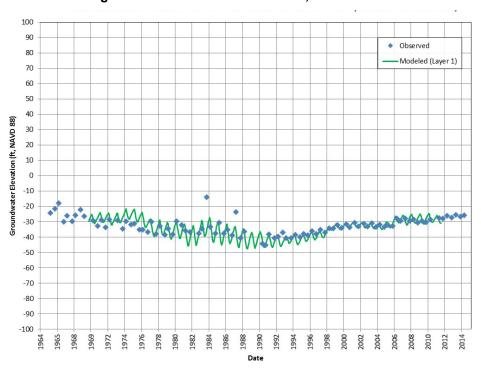
Figure 11i: Groundwater Elevation, Calibration Well 247
